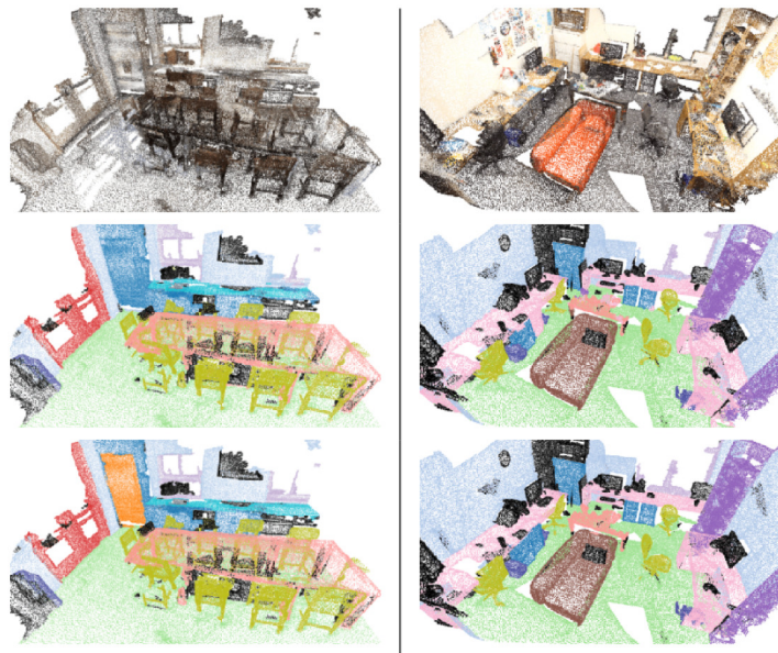
Figure 7: Visualization of Scannet predictions. From the top, a 3D input pointcloud, a network prediction, and the ground-truth.
